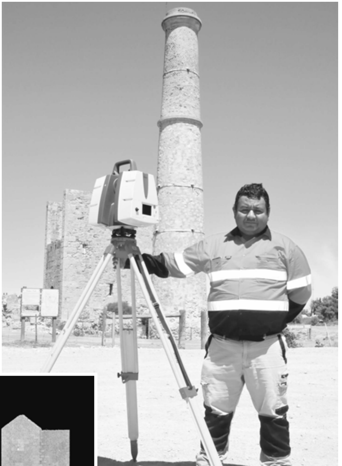
SURVEYING... Nelson Surveyors' Nelson Boquin demonstrates laser survey technology at Hughes Enginehouse, and inset, a copy of what the technology creates. The colour intensity can be switched on or off to identify movement in the structures, assisting with conservation works.
